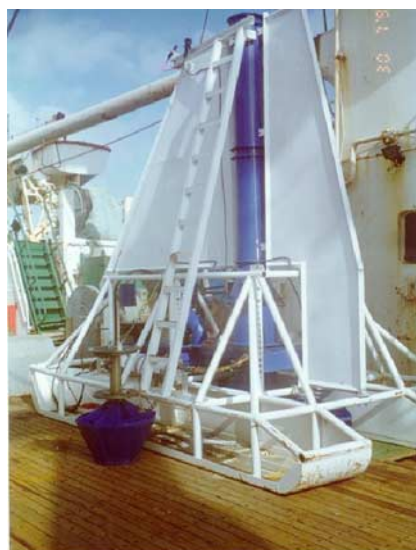
Fig. 5 Benthic disturber “deep-sea sediment re-suspension system” used for the experiment.
