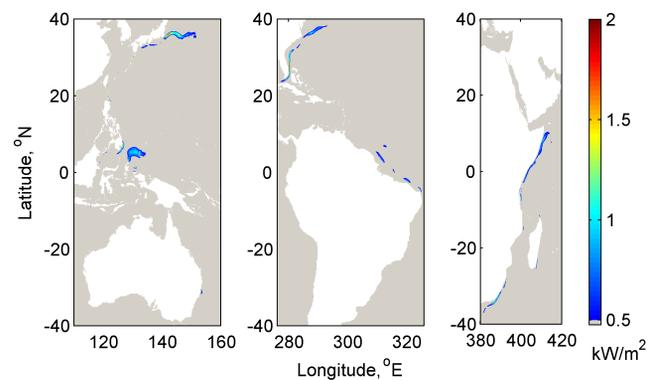
Fig. 1 HYCOM-calculated area with time-averaged power densities greater than  $0.5 \text{ kW/m}^2$  at 50 m depth (2009–2011) for the western boundary of the Pacific (left), Atlantic (center), and Indian (right) Oceans
