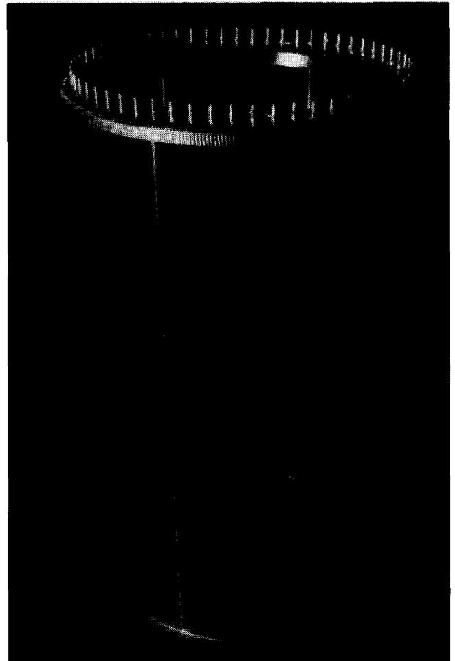
Fig. 1 Cage of nylon line ready for insertion in spin former
