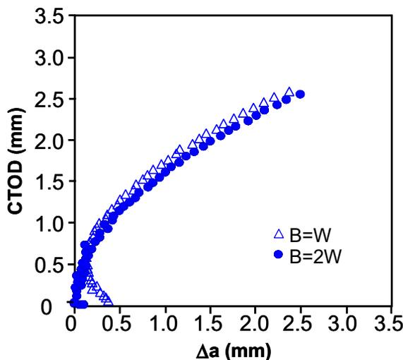
Fig. 3 Comparison of R-curves measured with 2 SENT specimen configurations:  $B = 2W$  configuration and  $B = W$  with side-grooves
