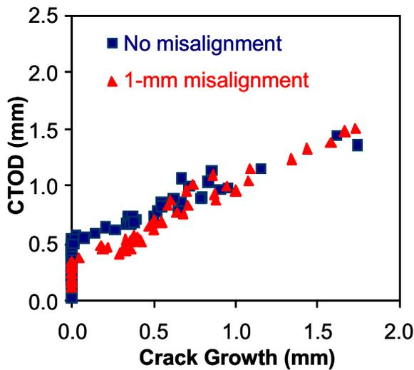
Fig. 2 Comparison of R-curves from two X65 full-scale tests with and without misalignment
