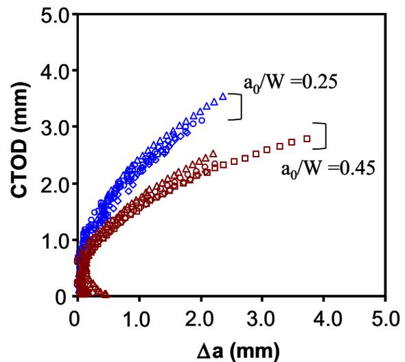
Fig. 4 Comparison of SENT R-curves extracted from pipe but with different  $a_0/W$  ratios
